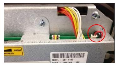
5c. Unscrew the two green grounding straps from both sides at the rear of the Monitor.
