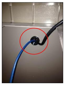
8d. The EPP Keypad Serial Connector should be attached to the port, labeled EPP, on the front of the Main Control Board.
