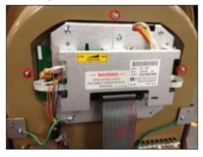
9b. Re-attach the green grounding straps on the left and right sides of the rear of the Monitor.
