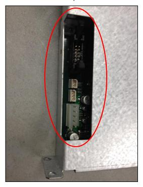
6c. The Main Control Board and metal housing is attached to the ATM with two screws at the rear base. Green grounding straps are attached at this same location. Remove the two screws (and retain). The Main Control Board and housing can now be lifted and removed.
