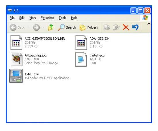
Notice that the 5 files are copied directly to the root of the SD card. They are not in a folder of any kind.
